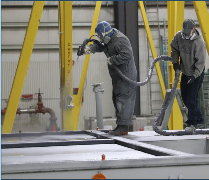
3. Factory trained material applicators, applying EFI spray-on coating to a skid station for Westmoreland, PA.
