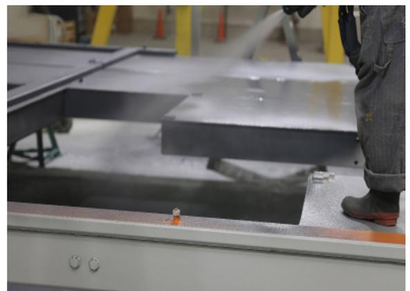
2. Factory trained material applicator applying EFI spray-on coating to a skid station for Westmoreland, PA.
